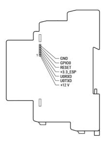
**△CAUTION!** High voltage on the add-on interface when the Device is powered!
